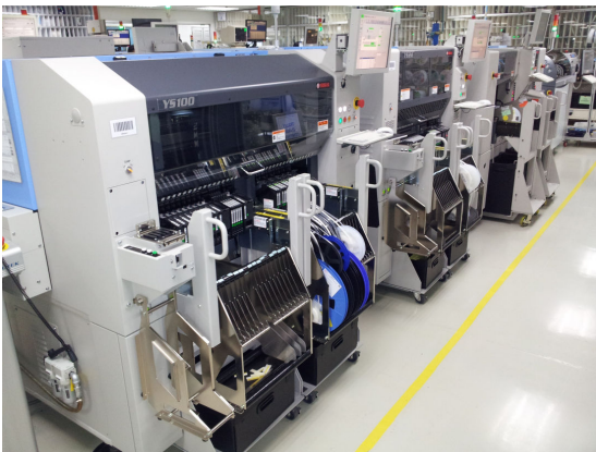
The new Yamaha YS100 pick and place machine on left and new moulding machines on right
